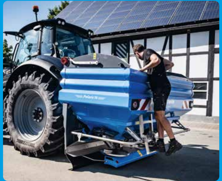
Roller tarp available in a mechanical or hydraulic version
