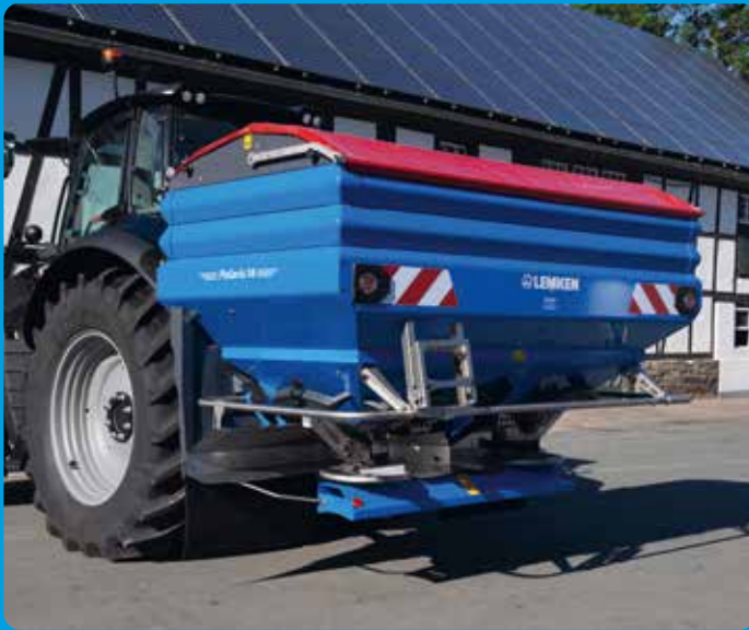
Hydraulic drive for constant disc speeds even on slopes
